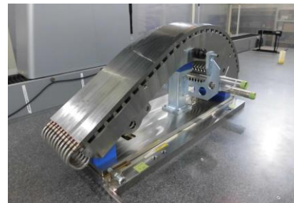
Diverter Left Outer Vertical Target prototype completed (March 2023)
